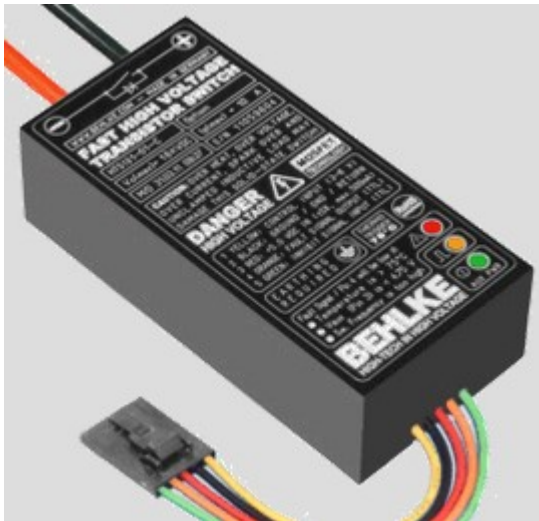
Figure 4: Behlke 33 kV 60 A MOSFET switch. Upper wires are HV inputs, lower are optoinsulated controls (Gate).
